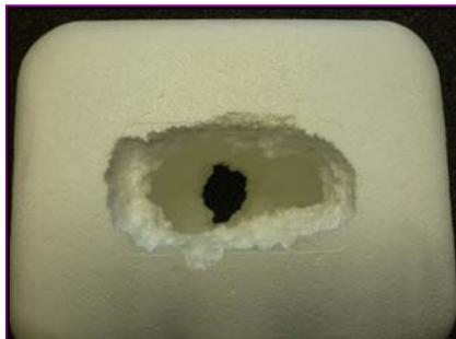
**Figure 3a: Fatty Acid Methyl Ester PCM on EPS Shipper - 10 minutes**
